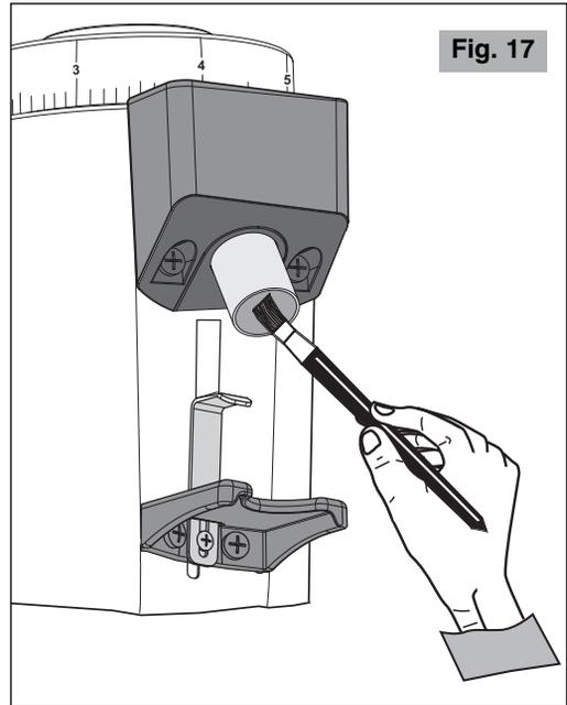
Once the hopper has been removed it can be washed with lukewarm water and neutral soap, then rinse it and dry well.
