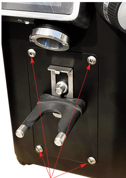
Unscrew the 4 screws of the module
